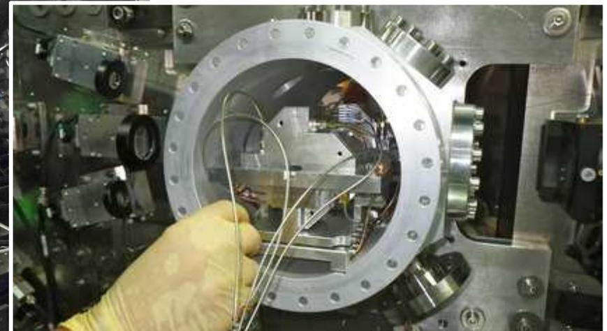
IP-BPM with mover in a vacuum chamber
