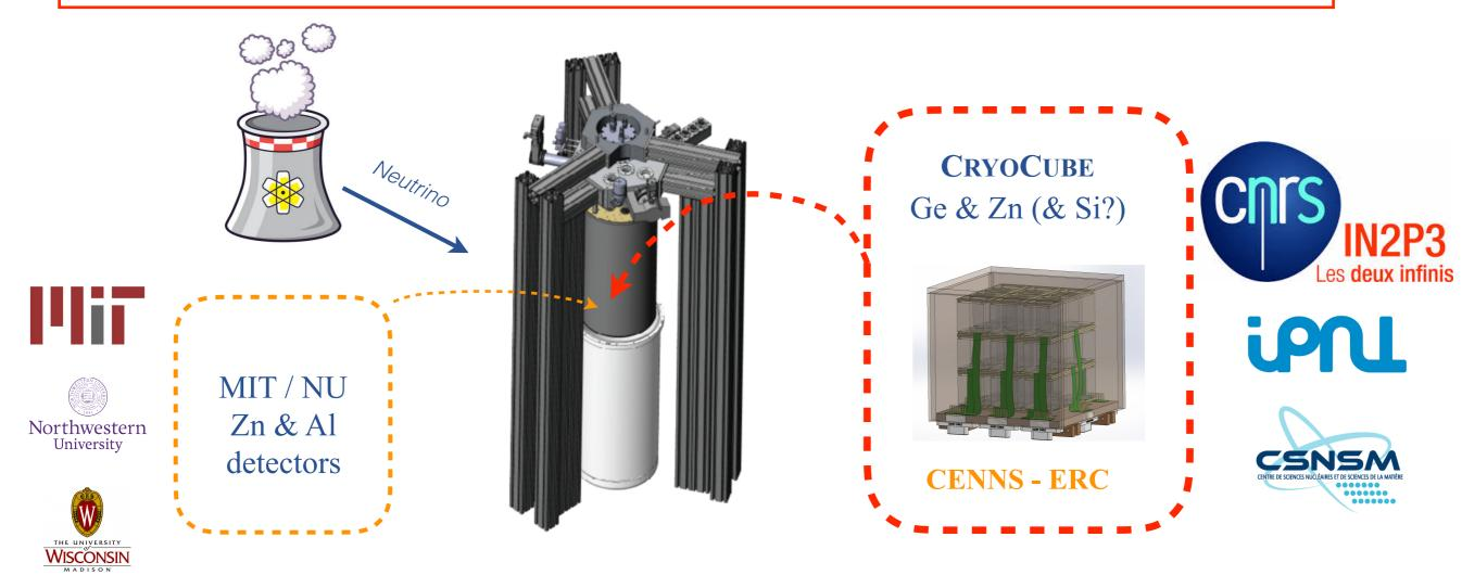
The CENNS - ERC will be funding the CryoCube **1kg of cryogenic Ge and Zn detectors with O(10) eV threshold and 10<sup>3</sup> rejection** RICOCHET is actively looking for new collaborators
