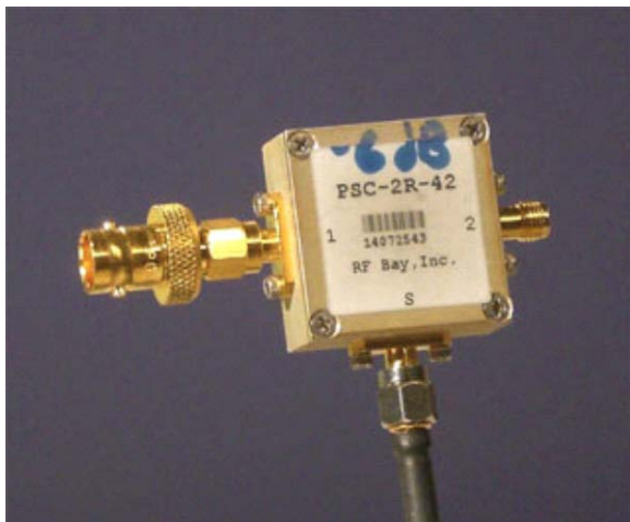
Figure 2 - This three-port splitter comes equipped with SMA connectors. The port on the left has an SMA-BNC adapter added to it.
