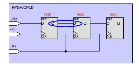
Simple synchronizer circuit between two asynchronous clock domains
