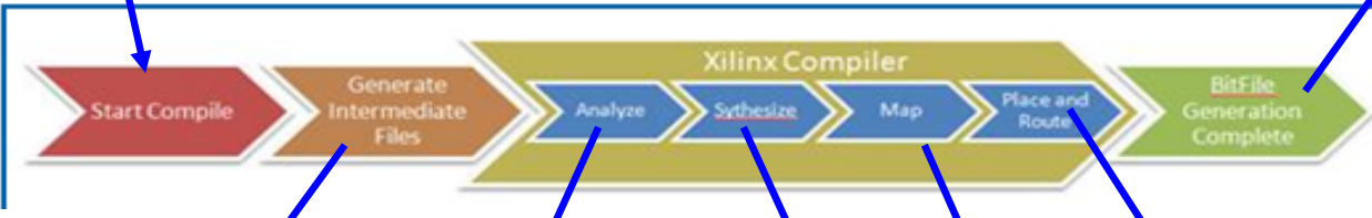
Figure 1. The Compile Process from Run Arrow to Bitfile
