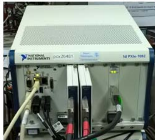
PXIe DAQ – 2 x FlexRIO boards
