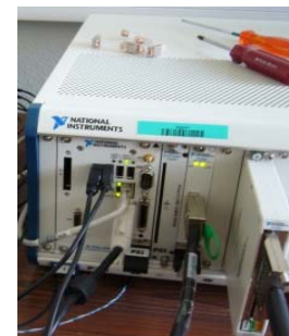
DAQ IPHC – NI Telescope EUDET PXIe - 1 Carte Flex RIO + NI6585
