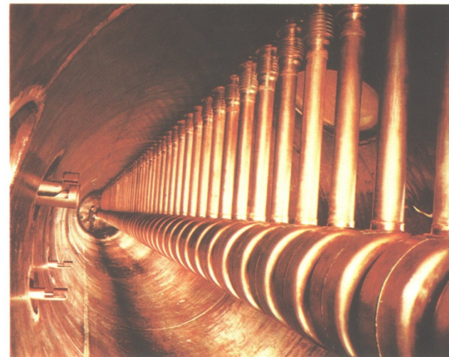
a drift tube linac (DTL) (Saturne, Saclay)
