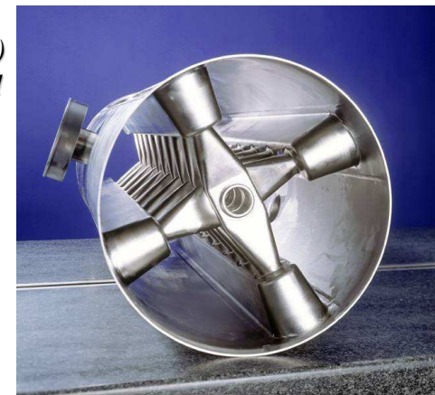
19-gap CH-DTL (Frankfurt) 350 MHz - \beta \sim 0,1
