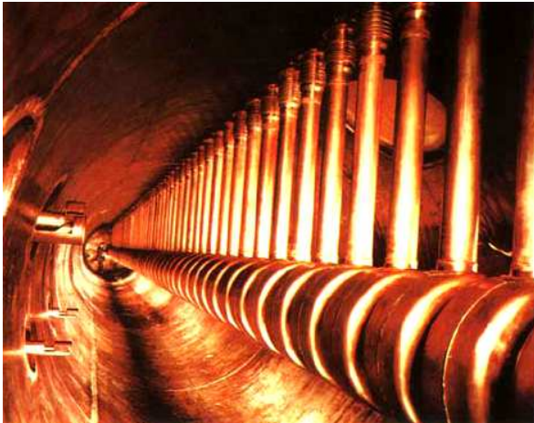
Saturne DTL (Saclay) : -> 20 MeV, 200 MHz
