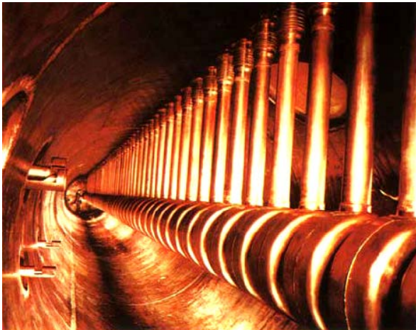
Saturne DTL (Saclay) : -> 20 MeV, 200 MHz
