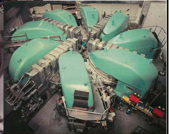
Cyclotron PSI (p, 590 MeV, 2mA, 50.6 MHz)
