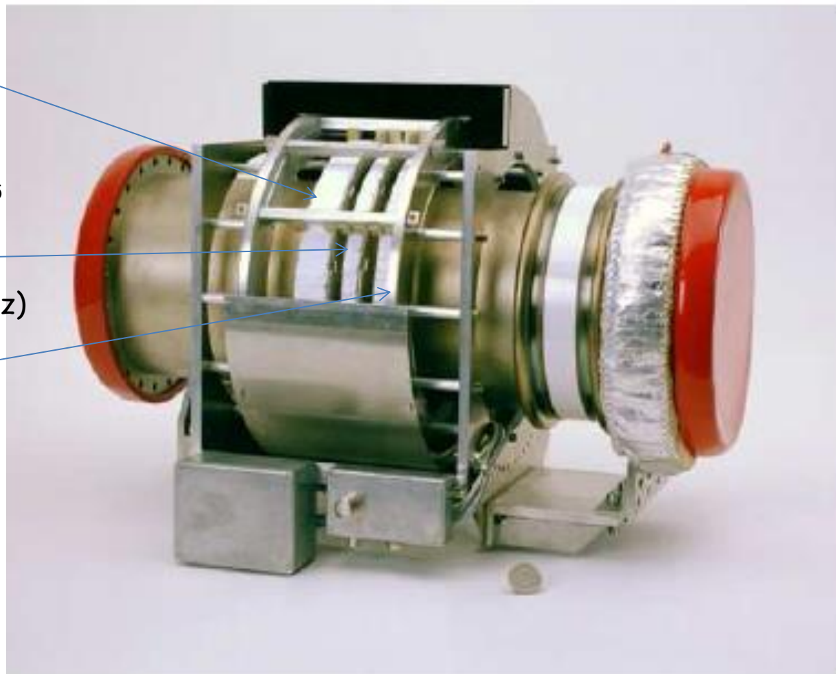
DC and AC Beam current transformer à GSI
