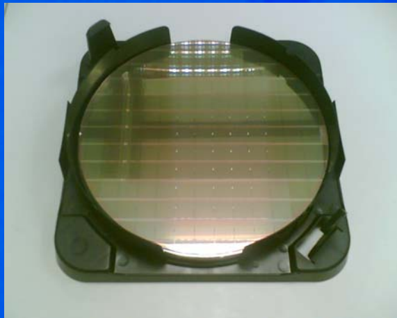
200mm wafer in its “wafer shipper” box, in the 250nm CMOS technology used for LHC
