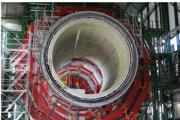
Figure 3 : CMS Detector : Superconducting coil in place at CERN in Geneva.
