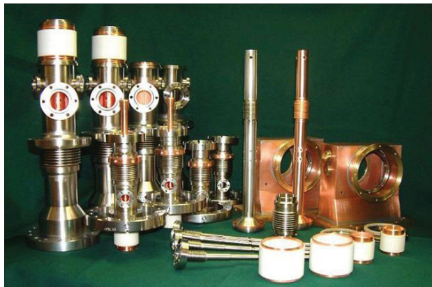
Figure 1 : Various parts of the XFEL TTF3 couplers which could be used for the ILC linear collider, including warm and cold assemblies, ceramic windows, wave-guide transitions and bellows.
