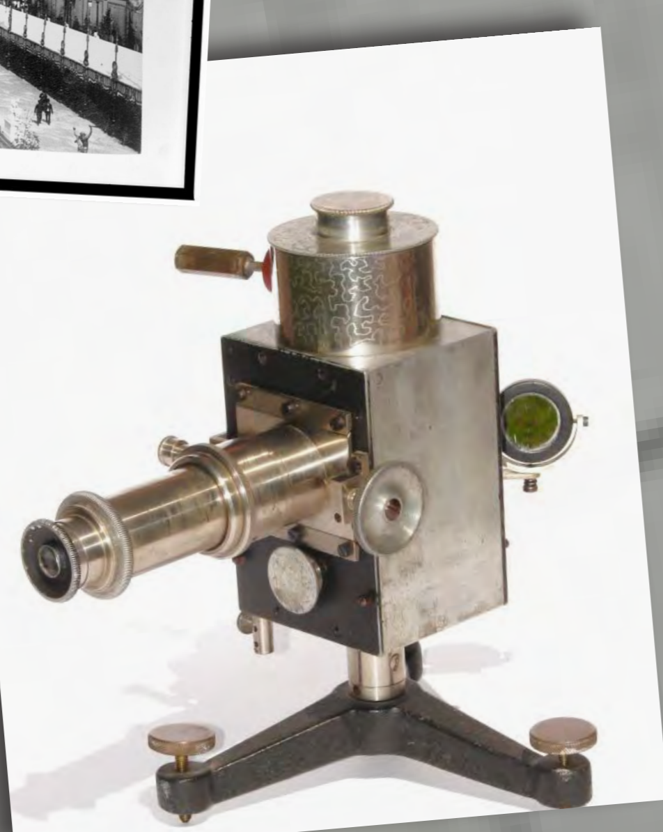
Electroscope de Wulf (1912) © University of Innsbruck
